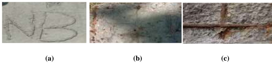
Figure-5 Bacterial concrete slab before and after 365 days of immersion in sea water
